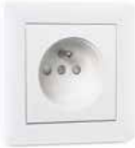
Çocuk Korunmalı Ups Priz * Socket-Outlet with Earthing Pin and Child Protection 65001053 16 A, 250 V~ IEC 60884-1
