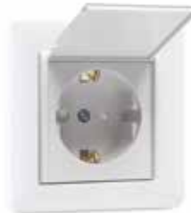
Çocuk Korunmalı Kapaklı Topraklı Priz * Earthed Socket-Outlet with Child Protection and Lid 65001254 16 A, 250 V~ IEC 60884-1
