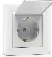
Çocuk Korumalı Kapaklı Topraklı Priz* Earthed Socket-Outlet with Child Protection and Lid 65001254 16 A, 250 V- IEC 60884-1
