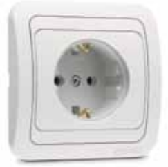
* Topraklı Priz Earthed Socket-Outlet 12028 16 A, 250 V~ IEC 60884-1
