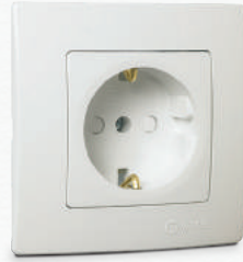
Çocuk Korumalı Topraklı Priz* Earthed Socket-Outlet with Child Protection 32001058 16 A, 250 V~ IEC 60884-1
